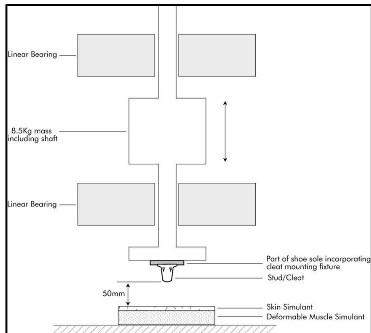
The test rig should stand on a rigid, high mass base to eliminate energy losses through vibration.
