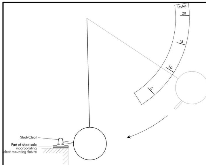
its side from the striker of a ballistic pendulum or similar device. The energy of the blows is increased in steps until either the stud/cleat or its means of attachment fails or a specified energy level is reached without damage occurring.
